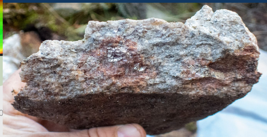
Mineralized Granite Assayed 7.38g/t Au Potassic and Carbonate Alteration
