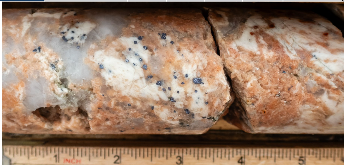
HML25-013 Box 29, 126.66m to 126.45m Mineralization Photo (4g/t Au over 2m from 125m interval)
