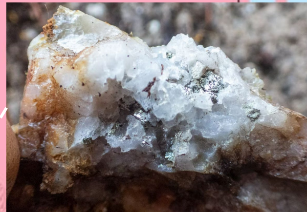
Quartz Vein and sulfide mineralization associated with pegmatites cutting through the granite intrusion
