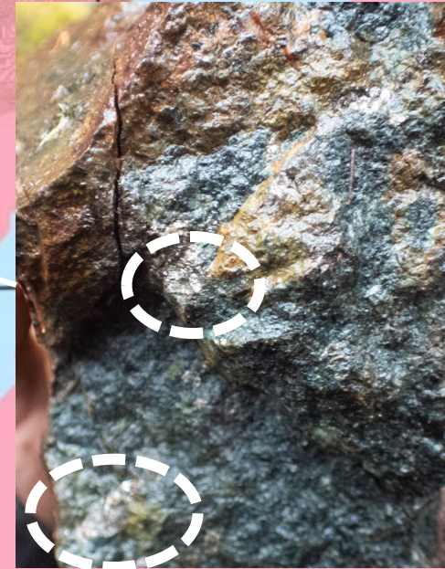
Mineralization in mafic volcanics (Arsenopyrite)
