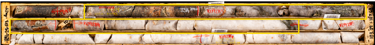
Figure 4: HML25-013 Box 24 (103.29m – 107.68m) 1.83 g/t Au from 103.5m
