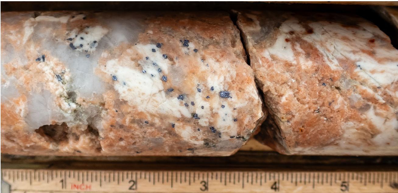
Figure 3: HML25-013 Box 29, 126.66m to 126.45m Mineralization Photo (4g/t Au over 2m from 125m interval)
